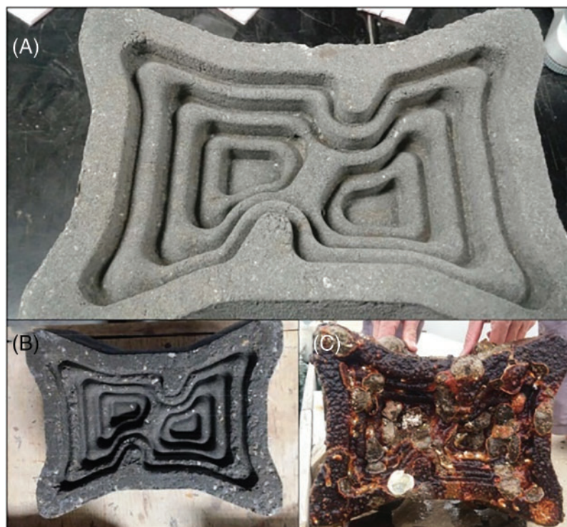
Fig. 5. ECO block samples: (A) Untested and brand new, (B) after enduring 75 freeze-thaw cycles for extreme weather conditions applications, (C) after being submerged for six months, adopted from Sella et al. [53].
